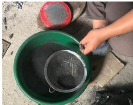
Image. Corn Cob Charcoal Filtering Process
