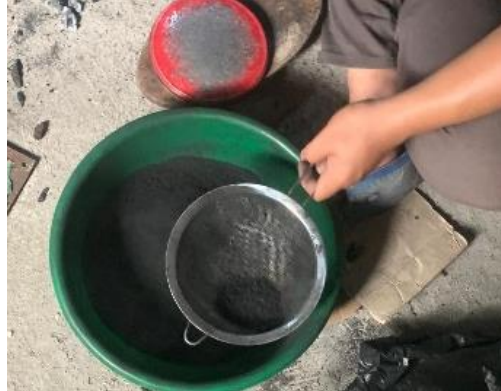
Figure 1. Corn Cob Charcoal Filtering Process
